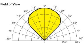
To meet the requirements of EN54:10 clause 5.4, where the ratio of the response points Dmax:Dmin should not exceed 1.41, the horizontal and vertical viewing angles  $\alpha$ max should not exceed  $\pm 30^{\circ}$
