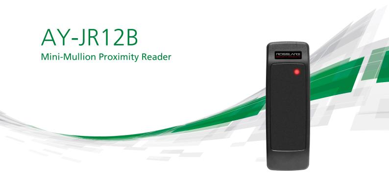
Rosslare's AY-JR12B is a powerful RFID proximity card reader of 125 KHz cards and tags, featuring Wiegand 26-Bit output format and a read range of up to 10 cm (3.9 in.). With a sleek design and a tough, UV-resistant and waterresistant casing, the AY-JR12B is equally suited to indoor and outdoor use and is both economical and reliable.
