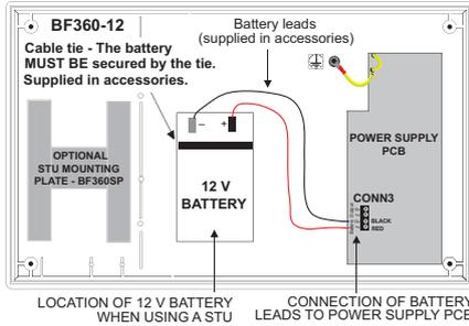
Position and connect 1 x 12 V battery (BF360-12), or 2 x 12 V batteries (BF360-24), as shown in the diagrams. Batteries must be safely secured using the supplied cable ties.
