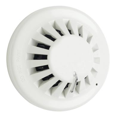
The conventional range offers a multi-mode, 5 in 1 detector (FXN922), covering many building needs. It's quick and simple to install with a stylish low profile design. The detector is mounted on our standard conventional base but can also be used in conjunction with our relay base for local switching. Each detector is fitted with a 360° viewable LED for indication.
